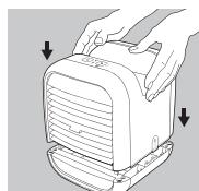
5. Replace the Top Cover onto the water reservoir.
