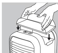
5. Place the tank into the MyChill cavity, making sure the tank is firmly seated. Water will begin to transfer into the water reservoir.
