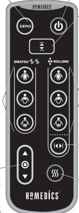
Power Button 🛈 - To turn on the unit, first press the POWER button. The LED indicator will illuminate and confirm your selection. To turn off the unit, simply press the button again. The LED indicator will blink while the back massage mechanism returns to its lowest point and then it will turn off.
